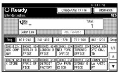
The list of programmed files being transmitted or waiting for transmission is displayed.
